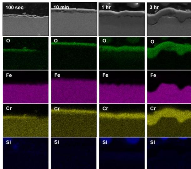
Fig. 7. EDS mapping results for the cross-sectional oxide images for Fe<sub>20</sub>Cr<sub>2</sub>Si after the oxidation testing
