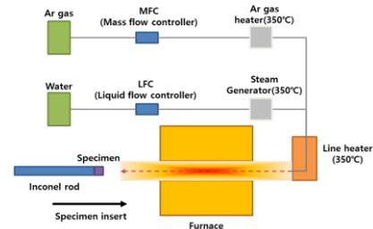
Fig. 1. Schematic of high temperature steam oxidation furnace
