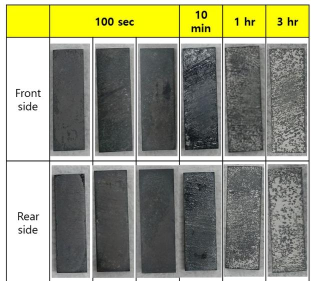
Fig. 5. Surface images of Fe<sub>20</sub>Cr<sub>2</sub>Si after the high temperature steam oxidation testing
