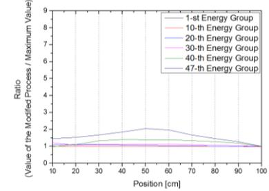
Fig.3 The ratio between the sum  $\psi_i^+(P) / R_i$  from the modified transport process and maximum  $\psi_i^+(P) / R_i$
