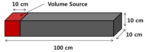
Fig. 1. Calculation model for a simple stick problem
