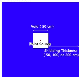
Fig. 5 Calculation model for the hollow cube problem
