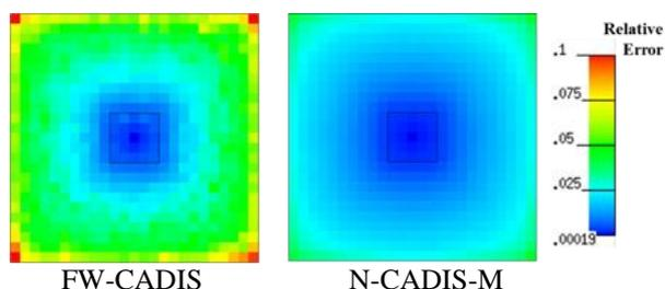
Fig. 6 The relative error distribution obtained by using the FW-CADIS and N-CADIS-M methods for the case of 100 cm shielding thickness problem
