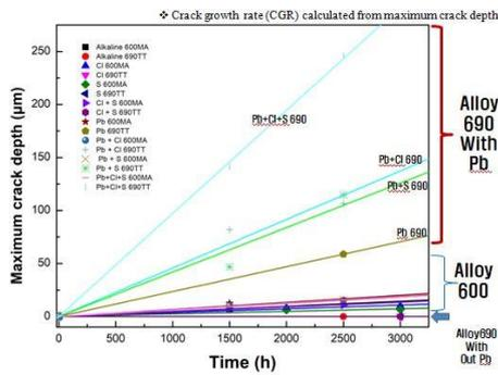
Fig. 1. Crack depth with immersion time for Alloy 600 and 690 in an experimental solution
