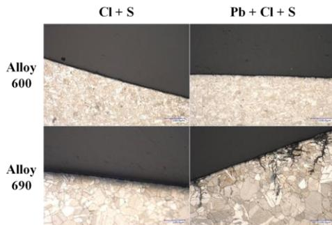
Fig. 2. Optical microscope images of Alloy 600 and 690 in Cl + S and Pb + Cl + S solutions.
