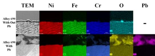
Fig. 3. STEM-HAADF images and EDX elemental maps obtained from APEX in Alloy 690 with and without Pb
