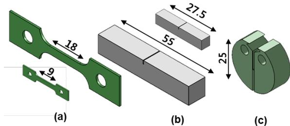
Fig 3. Specimen types and shapes for irradiation
