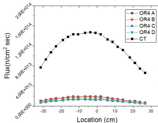
Fig 2. Flux distribution of OR4 irradiation hole and CT irradiation hole in Hanaro depending on axial position
