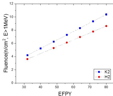
Fig 1. Estimated fluence level of Kori 2 and Hanbit 2 reactor vessels
