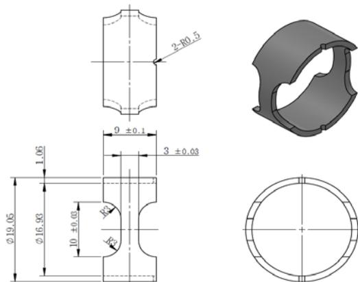
Fig. 1. Geometry of Ring-type circumferential specimen
