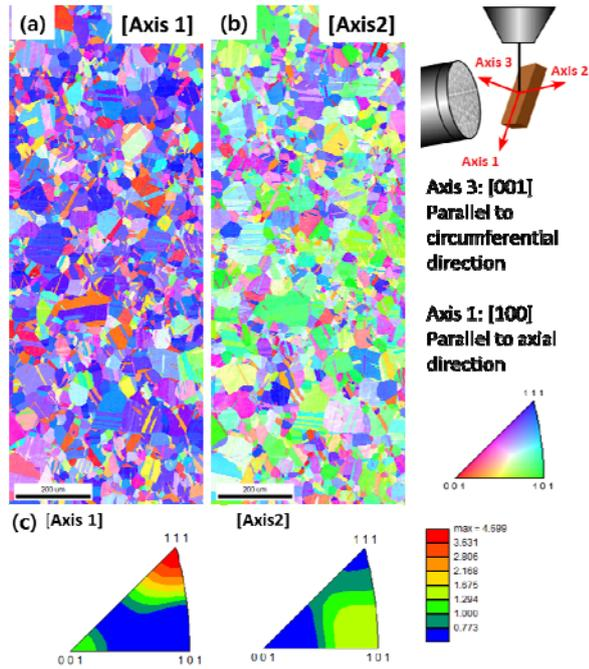
Fig 3. Inverse pole figure (IPF) map of Alloy 690 SG Tube measured to parallel to axial direction (a) and circumferential direction (b), and their IPF texture distribution (c)
