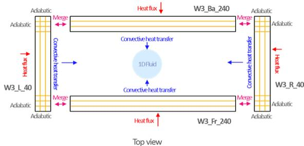
Fig 2. Modification of the boundary condition option of the GAMMA+ code
