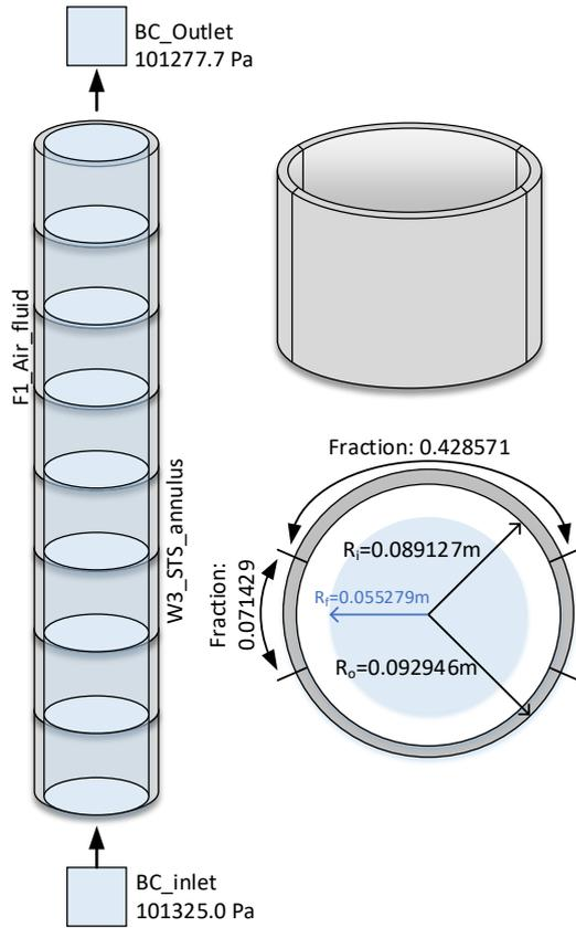
Fig 1. Riser modeling as a circular pipe in the extant version of the GAMMA+ code
