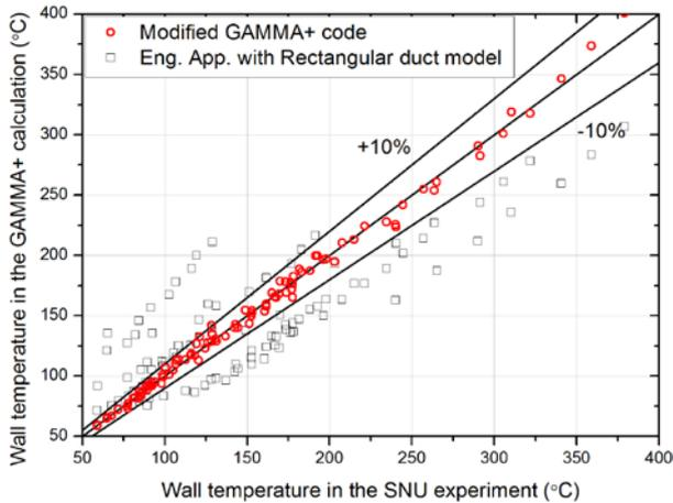
Fig 4. Calculation and comparison results for the SNU RHEF experiment
