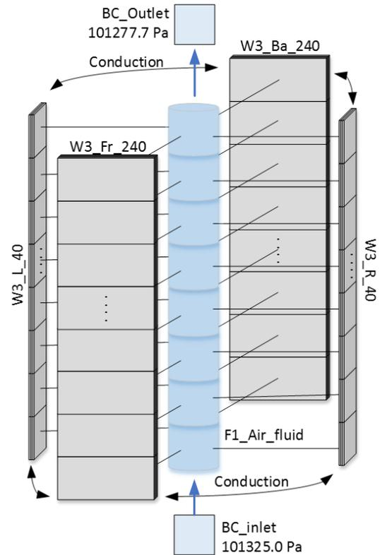
Fig 3. Riser modeling as a rectangular duct in the modified GAMMA+ code
