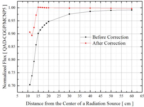
**Figure 2.** Correction Before and After Gamma-ray Flux Normalized by MCNP5 Results
