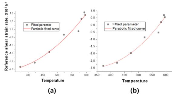
Figure 4. The obtained reference shear strain rate through the optimization code (dots) and the parabolic fitted line (red line) for (a) VPSC and (b) CPFEM.
