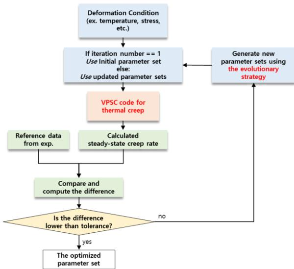
Figure 2. The schematic code flow used for optimizing parameters in VPSC model.
