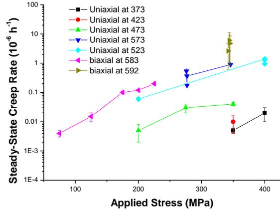
Figure 1. The axial steady-state thermal creep rates of the Zr-2.5wt%Nb pressure tube as a function of the applied stress from [1]
