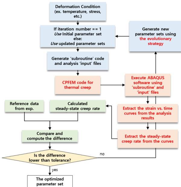
Figure 3. The schematic code flow used for optimizing parameters in CPFEM.
