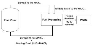
Fig. 2. Online-feeding process of dual fluid fusion-fission hybrid system.
