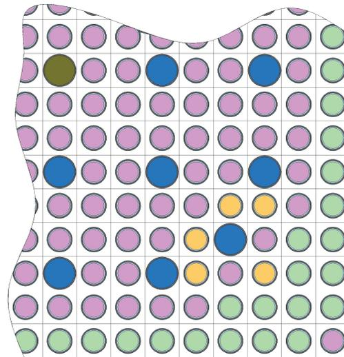
Fig. 1. FA design for Th-Pu SMR.
