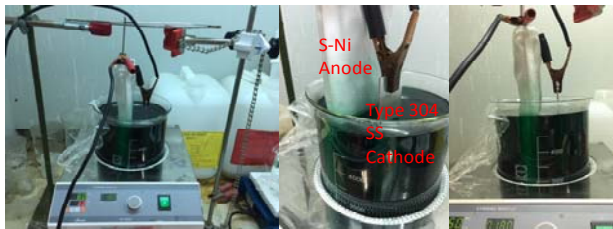
Fig. 4. Beaker test for setting up the Ni plating conditions.
