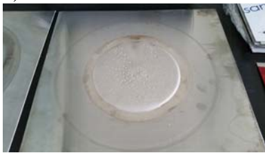
Fig. 1. Feature of plated Ni on type 304 stainless steel.
