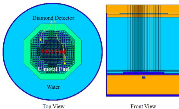
Fig. 1. Configuration of zero power CROCUS reactor.
