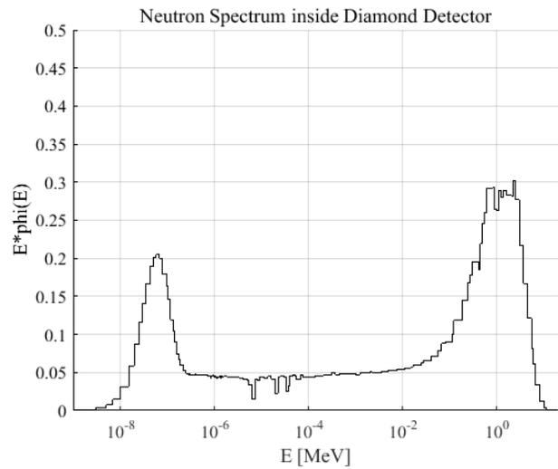
Fig. 2. Neutron spectrum in diamond detector.
