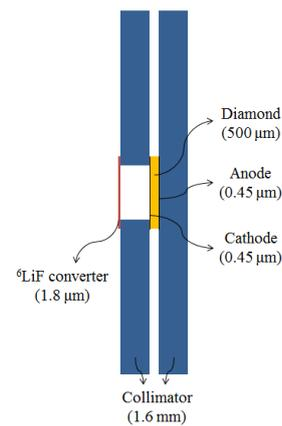
Fig. 3. Configuration of diamond detector.
