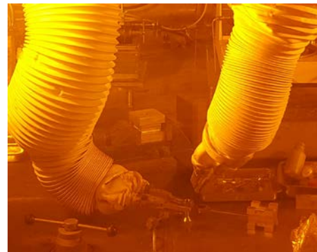
Fig. 3 Specimen assembling in Hot-cell
