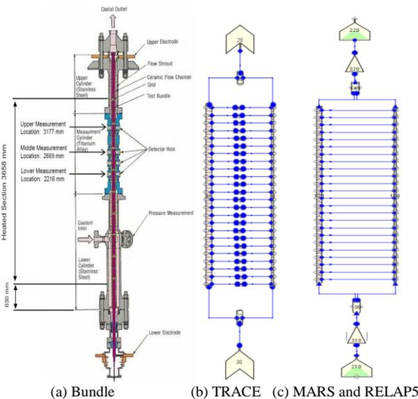
Fig. 2. Bundle test section and nodalization of each system code
