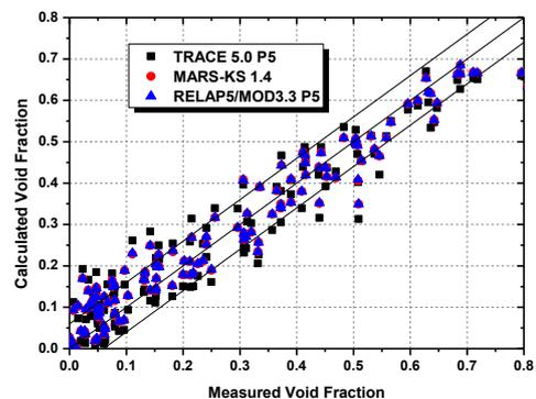
Fig. 4. Calculated void fraction results of call cases in single subchannel test
