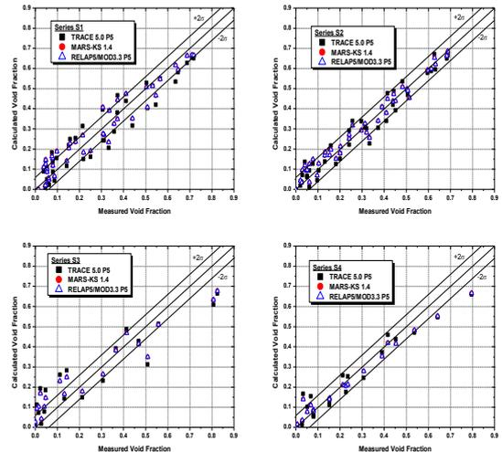
Fig. 3. Calculated void fraction results of each test series in single subchannel test
