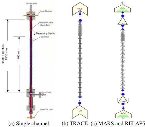
Fig. 1. Single channel test section and nodalization of each system code
