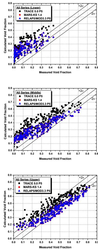
Fig. 6 Calculated void fraction results of all cases distinguished by measuring points
