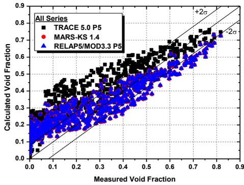
Fig. 7 Calculated void fraction results for all test series
