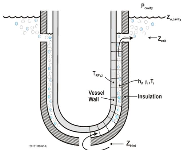
Fig. 1. Nodalization in cooling channel
