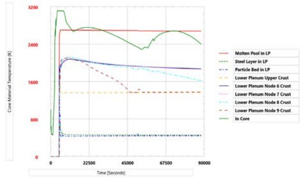
Fig. 3. Core Material Temperature Distribution for LBLOCA Sequence
