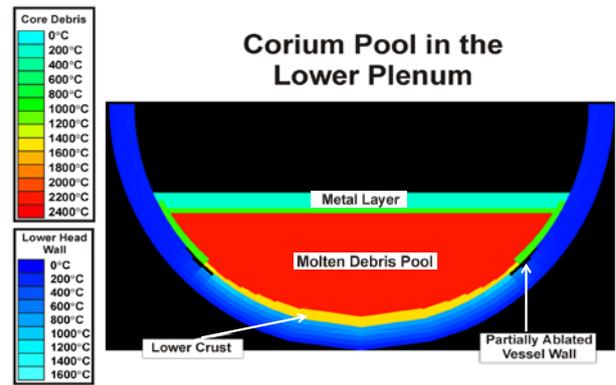
Fig. 4. Corium pool in the lower plenum at the end of run for LBLOCA Sequence
