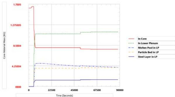
Fig. 2. Core Material Mass Distribution for LBLOCA Sequence
