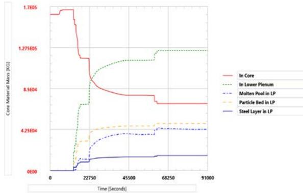
Fig. 6. Core Material Mass Distribution for TLOFW Sequence
