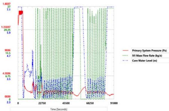
Fig. 7. In-Vessel Injection Conditions for TLOFW Sequence
