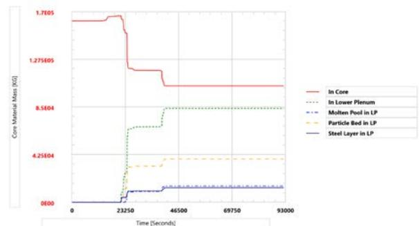
Fig. 5. Core Material Mass Distribution for SBLOCA Sequence
