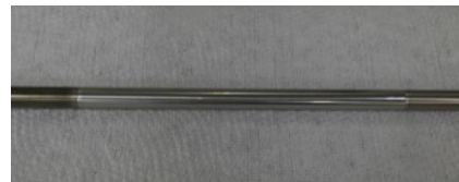
Fig. 1. Cr-alloy coated Zircaloy-4 by CAIP.
