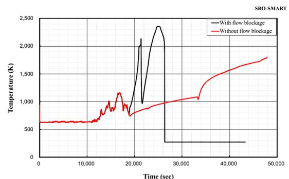
Fig. 2. Comparison of fuel temperatures (centering at 4/5 elevation) between the models with (reference) and without flow blockage.
