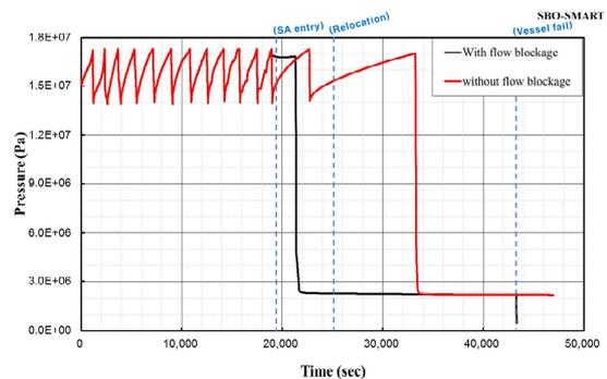
Fig. 1. Comparison of the primary pressures between the models with (base case) and without flow blockage.
