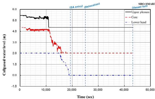
Fig. 3. Water level in the vessel.
