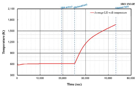
Fig. 5. Wall temperature of lower head.
