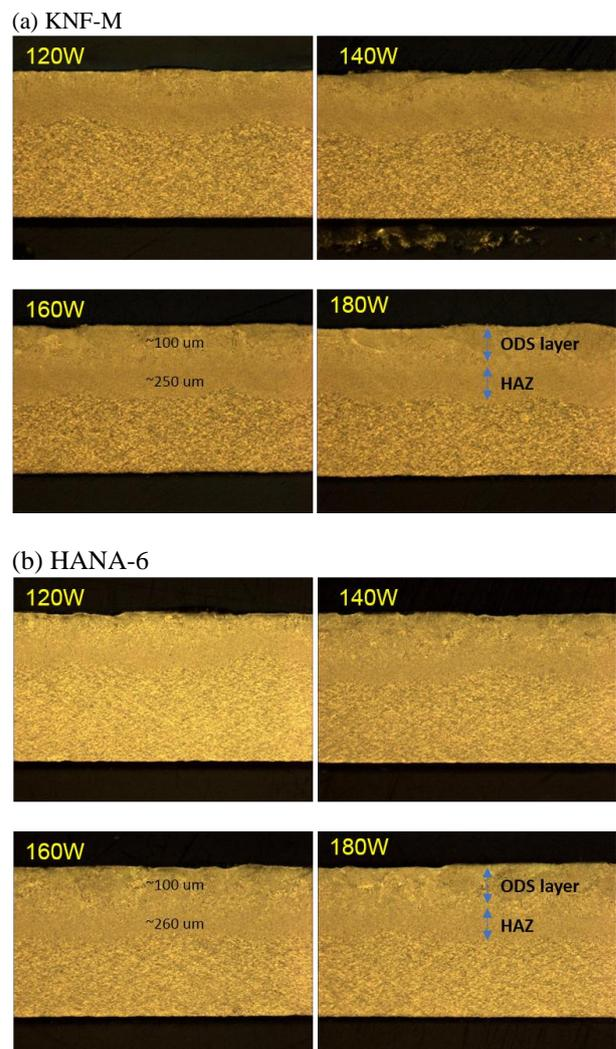
Fig. 3. Cross-sectional microstructures of ODS treated (a) KNF-M and (b) HANA-6 samples.
