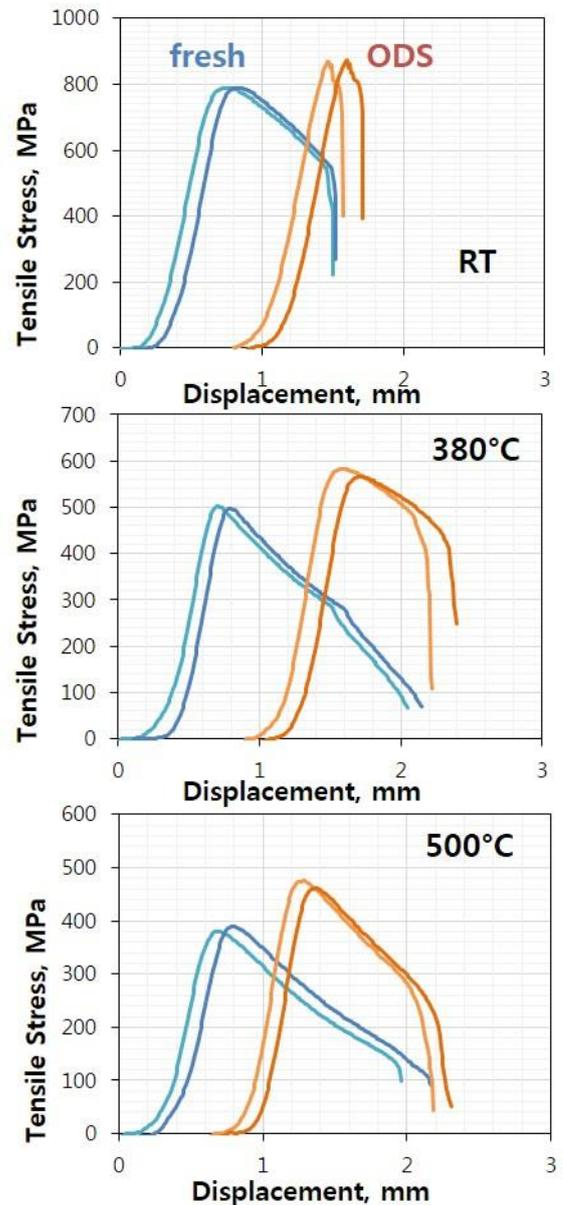
Fig. 6. Stress-strain curves of fresh and ODS Zircaloy-4 samples in ring tensile tests at room temperature (RT), 380°C, and 500°C, respectively [6].
