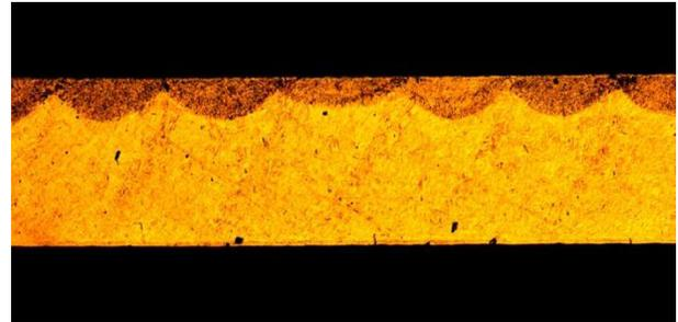
Fig. 2. Cross-sectional microstructures of ODS Zircaloy-4 samples showing the ODS layer formed at the surface.
