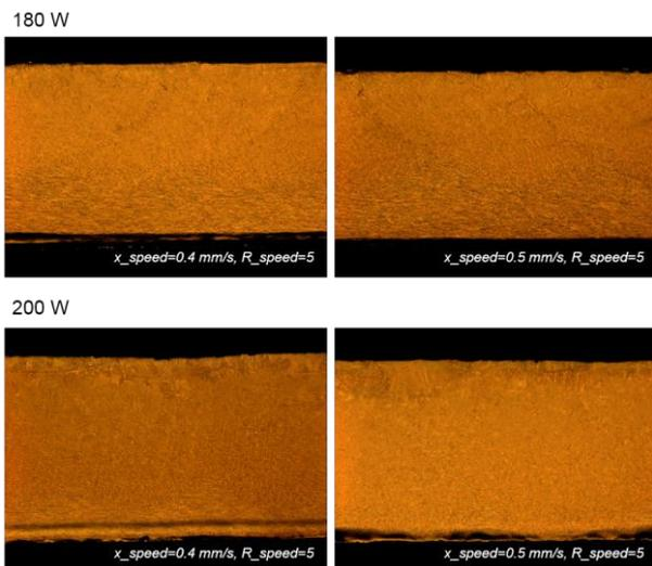
Fig. 5. Cross-sectional microstructures of ODS treated Zircaloy-4 samples using a laser with a 1 mm beam diameter.
