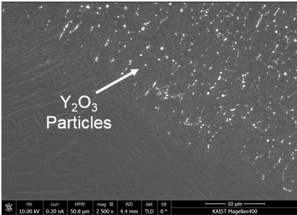
Fig. 4. SEM micrographs of ODS layer in HANA-6 samples.
