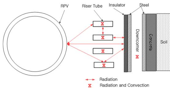
Fig. 2 RPV and the Air-Cooled RCCS Model of a 10MW<sub>t</sub> HTGR
