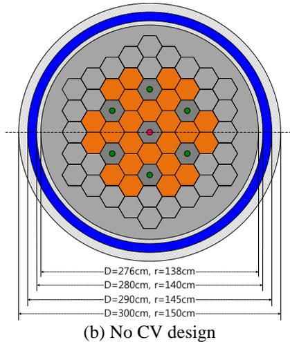
Fig. 1 Core Design of a 10MW<sub>t</sub> HTGR
