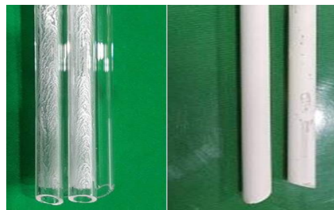
Fig. 3. Slurry brushing photos of quartz tubes obtained after sandblasting (left: without sandblasting, right: with sandblasting).
