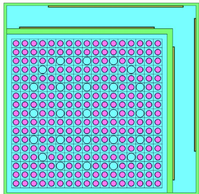
Fig. 2. Configuration of the basket cell of MPC-24
