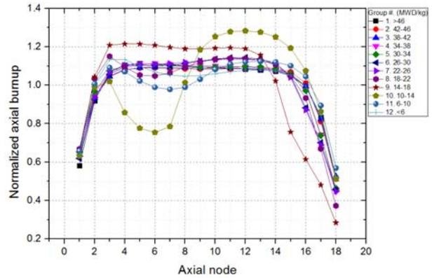
**Fig. 3.** Bounding axial profiles by burnup group
