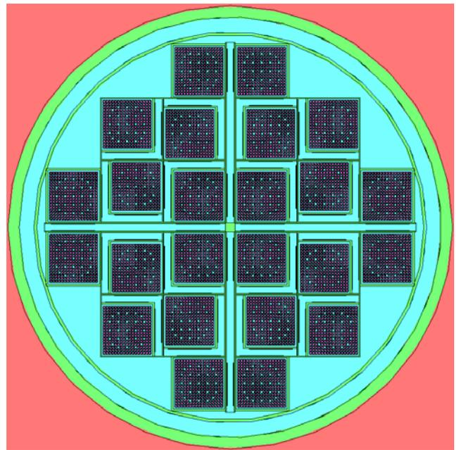
Fig. 1. Configuration of the HI-STORM 100 cask
