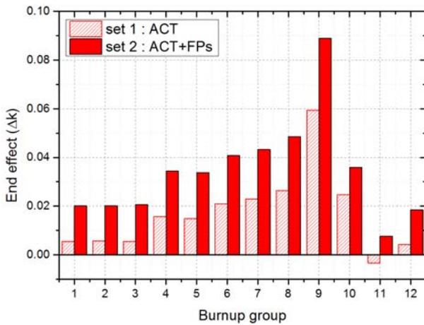
Fig. 4. End effect by applying the bounding axial profiles corresponding a fixed burnup of 40 MWD/kg
