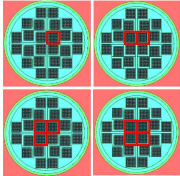
Fig. 6. Configuration of the misloading cases
