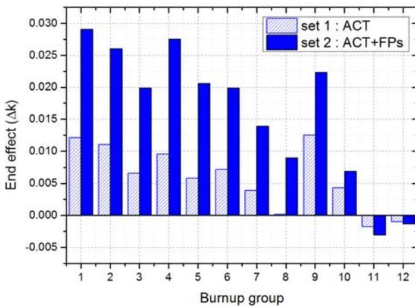
Fig. 5. End effect by applying the bounding axial profiles corresponding burnup group
