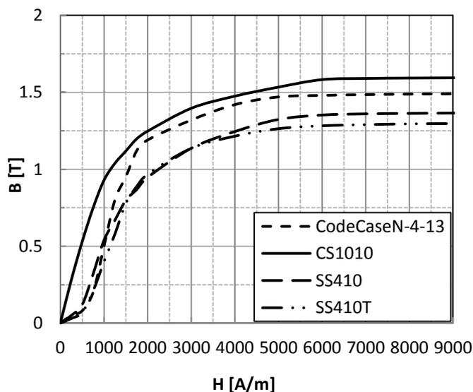
Fig. 2. Material B-H Curve
