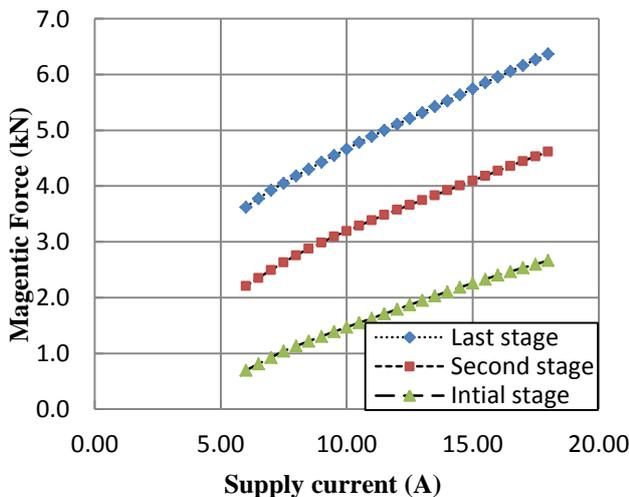
Fig. 5. Lifting force estimation at each stage
