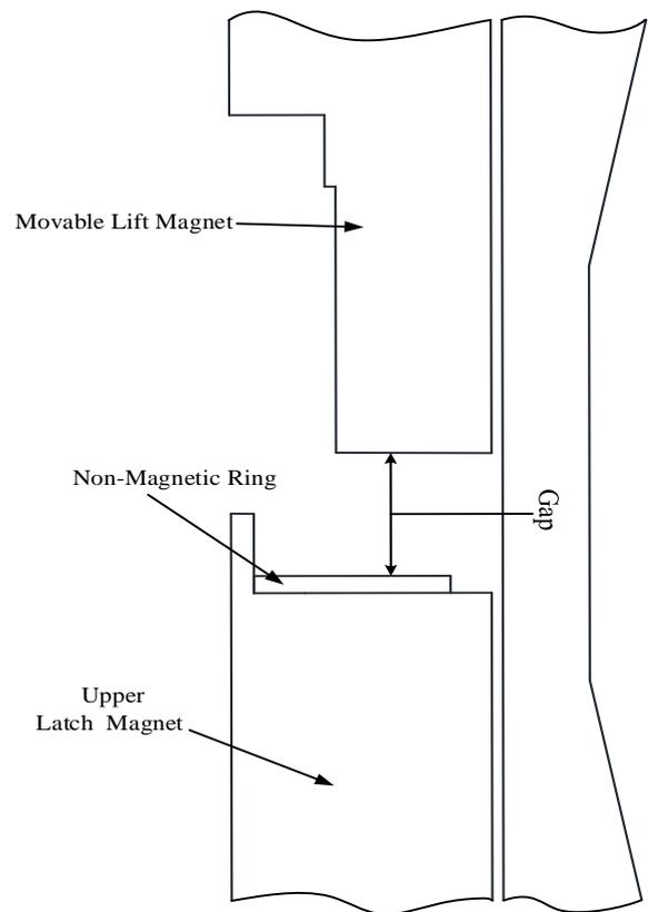
Fig. 4. View of Detail A
