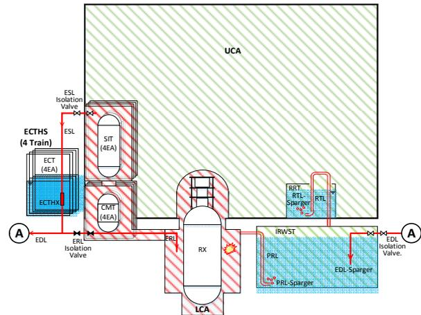
Fig. 1 Conceptual view of containment pressure and radioactivity suppression system(CPRSS) for SMART
