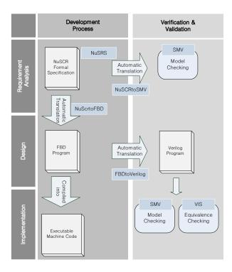
Fig. 1. Development process for NPP's software
