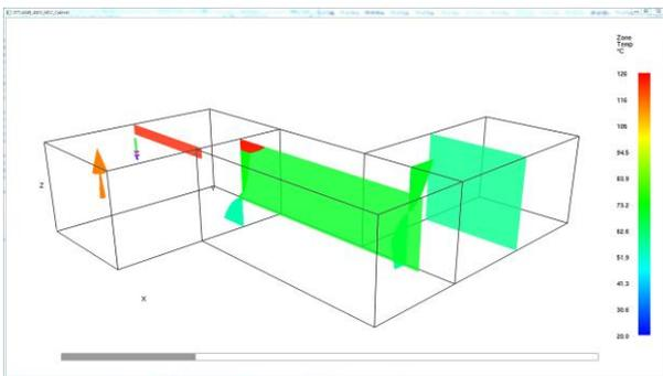
Fig. 2. CFAST/Smokeview Rendering for Fire Scenario of HVAC Equipment Room B.
