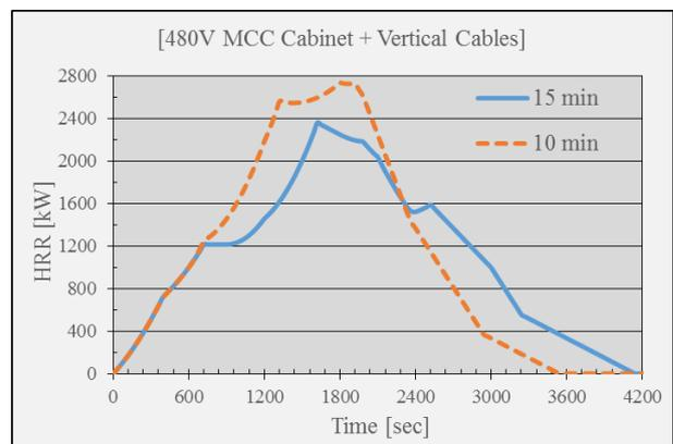
Fig. 4. HRR Profile of Initial Fire in 480V MCC Cabinet Set #1 and Vertical Cable Trays Depending on Time to Fire Propagation to Adjacent Cabinets (Peak HRR = 702 kW)
