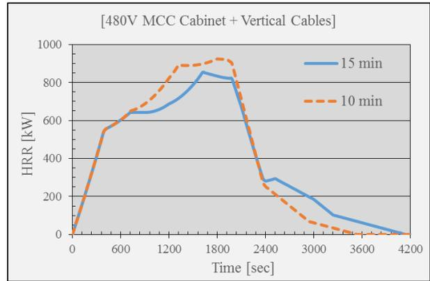
Fig. 3. HRR Profile of Initial Fire in 480V MCC Cabinet Set #1 and Vertical Cable Trays Depending on Time to Fire Propagation to Adjacent Cabinets (Peak HRR = 130 kW)
