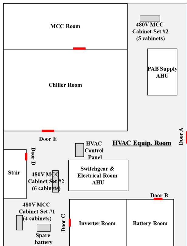
Fig. 1. Floor Plan of HVAC Equipment Room B.
