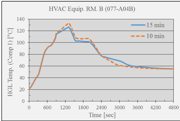
Fig. 5. HGL Temperature Profile in modeling compartment #1 of HVAC Equipment Room B Depending on Time to Fire Propagation to Adjacent Cabinets (Peak HRR = 130 kW)
