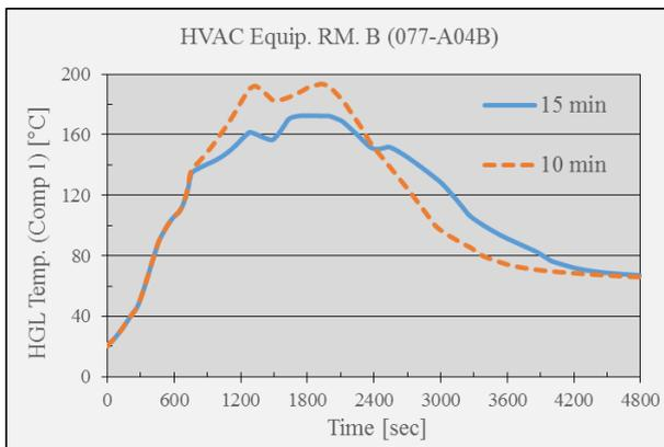
Fig. 6. HGL Temperature Profile in modeling compartment #1 of HVAC Equipment Room B Depending on Time to Fire Propagation to Adjacent Cabinets (Peak HRR = 702 kW)
