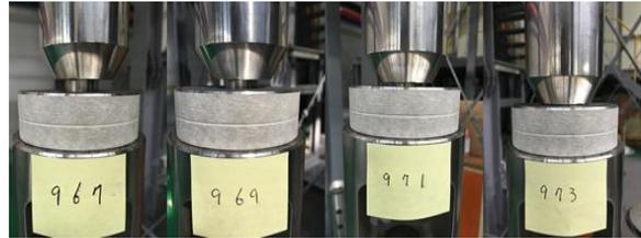
Figure 10 CRA gripper tests according to overlap distances between gripper and CRA head
