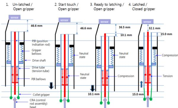
Figure 9 Bellows movement status during CRA gripper operation
