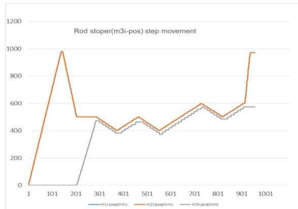
Figure 11 Step movements of rod stop system stopper for following the drive shaft
