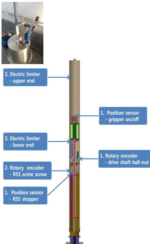
Figure 4 CRDM sensor system
