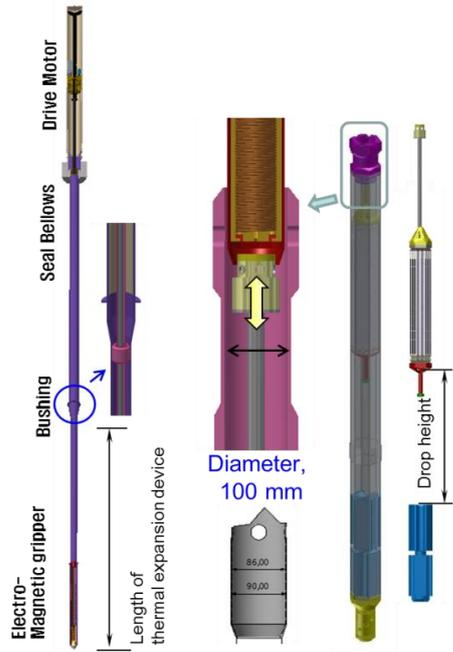
Figure 3 Secondary control rod drive system with passive shutdown device
