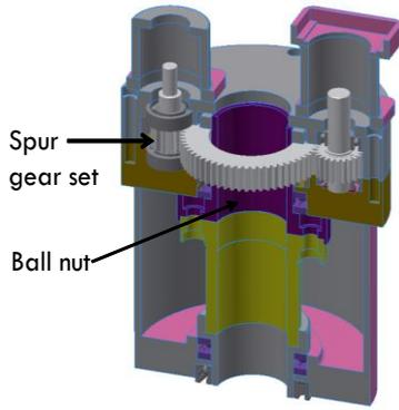
Figure 6 Drive motor spur gear set
