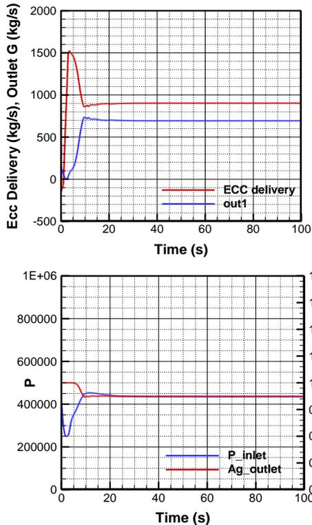
Fig. 2. ECC delivery and downcomer pressure transient.
