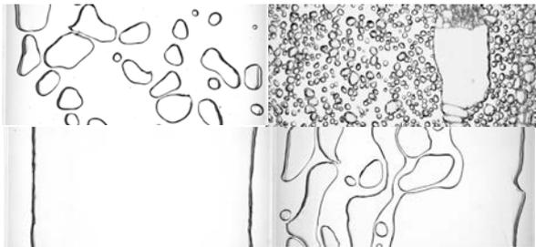
Fig. 3. Downward flow patterns (From top, left to right) (a) Large-bubbly flow at  $J_L = 0.8$  m/s,  $J_G = 0.4$  m/s, (b) Cap bubbly flow at  $J_L = 2.3$  m/s,  $J_G = 1.7$  m/s (c) Falling film flow at  $J_L = 0.3$  m/s,  $J_G = 0.0$  m/s, and (d) undefined flow at  $J_L = 0.4$  m/s,  $J_G = 0.6$  m/s
