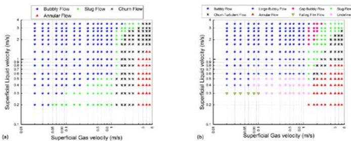
Fig. 4. Flow regime map for (a) vertical upward flow and (b) vertical downward flow in rectangular 2.35 mm test section
