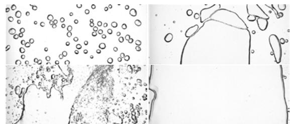
Fig. 2. Upward flow patterns (From top, left to right) (a) Bubbly flow at  $J_L = 1.3$  m/s,  $J_G = 0.3$  m/s, (b) Slug flow at  $J_L = 0.4$  m/s,  $J_G = 0.8$  m/s, (c) Churn flow at  $J_L = 2.0$  m/s,  $J_G = 2.5$  m/s, and (d) Annular flow at  $J_L = 0.3$  m/s,  $J_G = 6.0$  m/s
