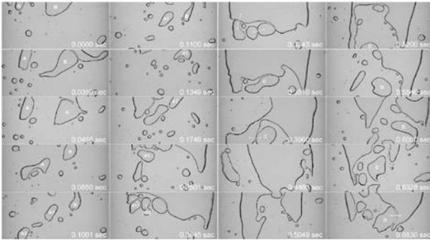
Fig. 6. Large-bubbly flow snippets at mentioned time intervals. Air bubbles, in this case, A, B, C and D remaining relatively stationary in the field of view. Bubble A is seen to be breaking into bubbles A1 and A2. Arrows indicate the forthcoming merger of two
