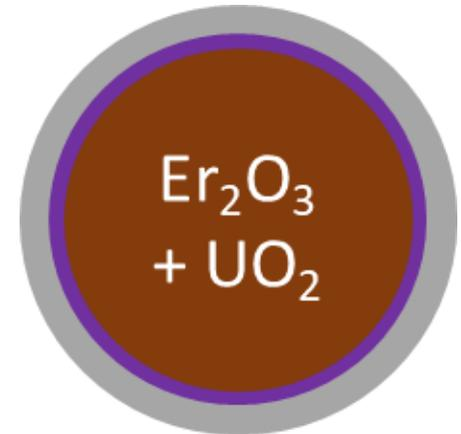
$\text{Er}_2\text{O}_3$ - $\text{UO}_2$  fuel pellet
