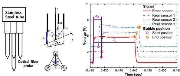
Fig. 1. The four-sensor optical fiber probe (Left: Design of 4S-OFP, Right: Typical bubble signal)
