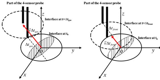
Fig. 3. Diagram of a bubble passing sensors of the probe
