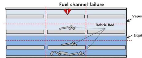
(b) Fuel channel failure & debris bed formation
