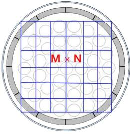
Fig. 2 Node system for a fuel channel in CAISER
