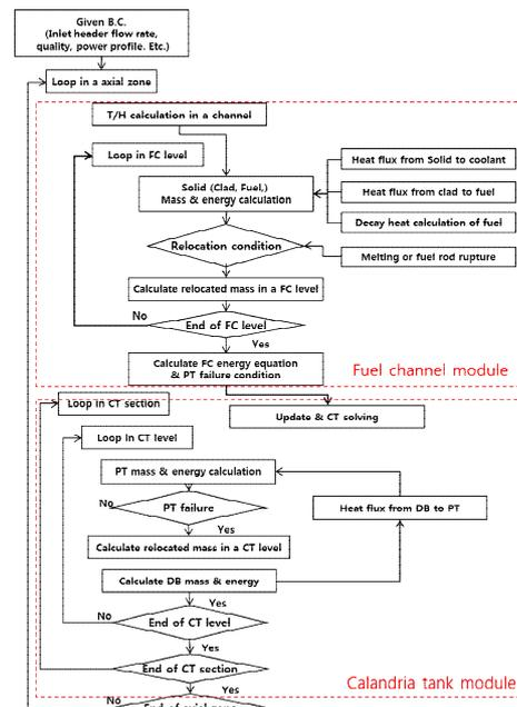
Fig. 5 Logic diagram for core degradation in CAISER
