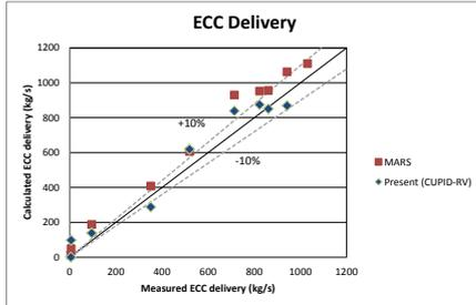
Fig. 7. Comparison of ECC delivery mass flow rate between CUPID-RV and MARS.
