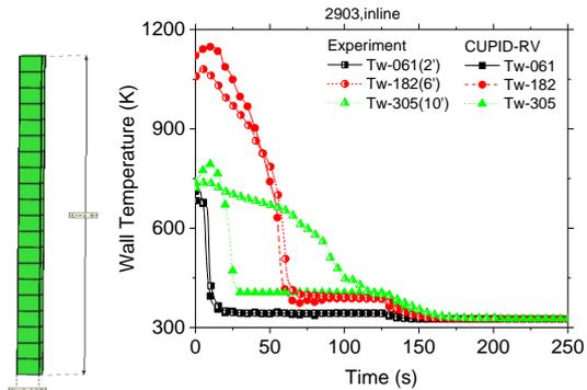
Fig. 5. Comparison of wall temperature transient between CUPID-RV and experiments.
