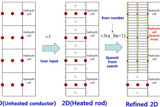
Fig. 3 Rezoning concept for reflood model
