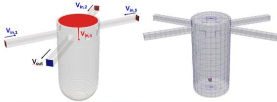
Fig. 6. UPTF test concept and calculation mesh.
