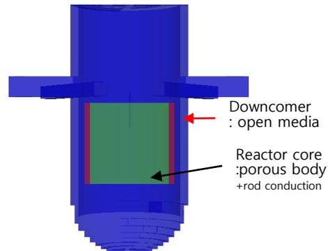
Fig.1 Concept of CUPID-RV module
