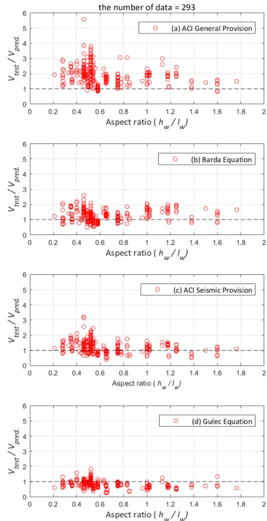
Fig. 1. Test strength divided by shear equations versus aspect ratio using a database with 293 flanged walls
