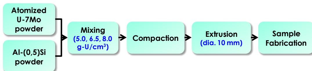
Fig. 1. A schematic showing sample preparation
