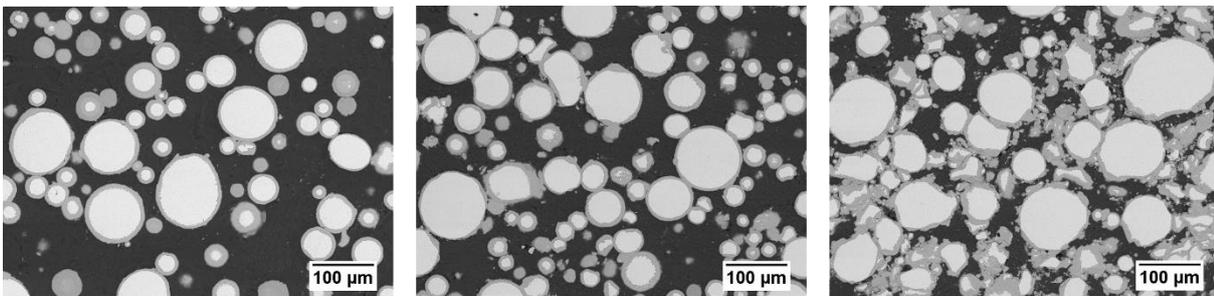
**Fig. 3.** SEM images of heat-treated U-7Mo/Al dispersion fuels at 530 °C for 8 hours: (a) 5.0 g-U/cm<sup>3</sup>, (b) 6.5 g-U/cm<sup>3</sup>, and (c) 8.0 g-U/cm<sup>3</sup> [7].
