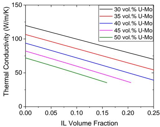
Fig. 6. Thermal conductivity of U-Mo/Al dispersion fuels as a function of IL volume fraction.
