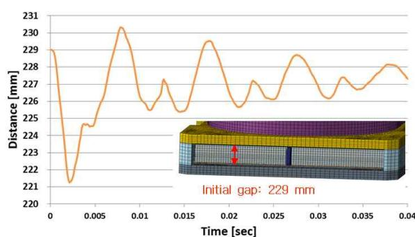
Fig. 4. Residual deformation of upper mechanism housing
