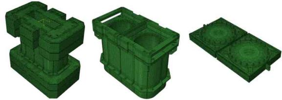
Fig. 2. Structural analysis model of high capacity CANDU spent fuel transport cask
