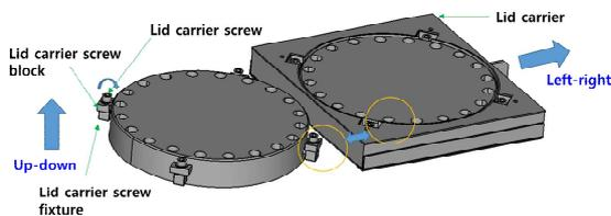
Fig. 1. Upper mechanism of high capacity CANDU spent fuel transport cask
