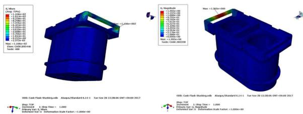
Fig. 3. Stress contour applied static stacking load to upper mechanism
