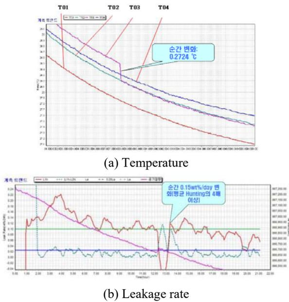
Figure 2 Trend of temperature and leakage rate
