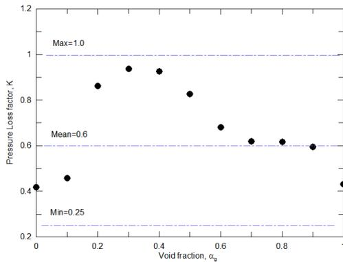
Fig. 4. Calculated k-factor at nozzle and uncertainty range
