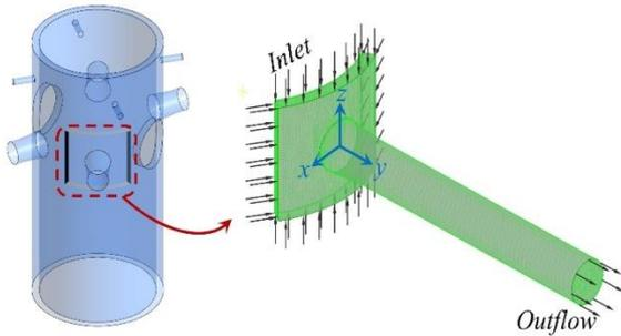
Fig. 3. Computational domain and grid system-
