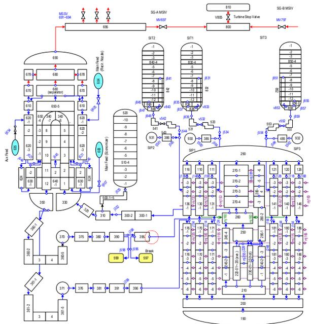
Fig. 5. MARS-KS nodalization for LBLOCA of APR1400
