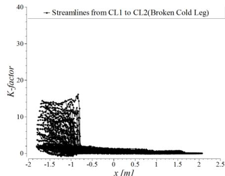
Fig. 2. K-factor along streamlines from cold leg 1 to cold leg 2
