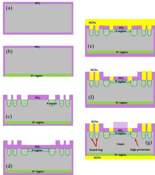
Fig. 1. Schematic of fabrication process flows of Si PIN photodiode: (a) Initial oxidation, (b)  $\text{POCl}_3$  doping on back side, (c)  $^{11}\text{B}$  implantation for an edge protection structure, (d)  $\text{BF}_2$  implantation for a shallow active area and oxidation, (e) Al/Au deposition on front side, (f) Lift-off of an active area, and (g) Al/Au deposition on back side.
