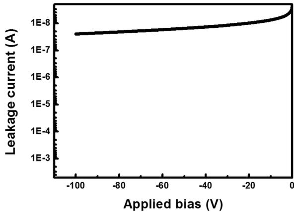
Fig. 2. Leakage current density as a function of the reverse bias voltage for a single Si PIN photodiode.
