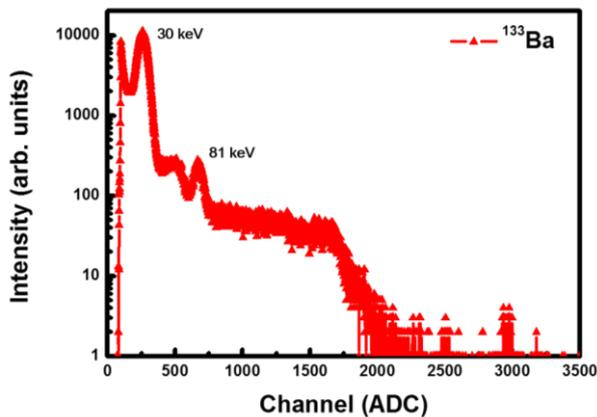
Fig.3. The pulse height spectrum of the Si PIN photodiode radiation detector measured using <sup>133</sup>Ba source.
