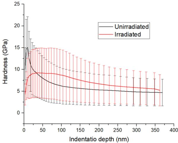
Fig. 2. Difference in hardness of Pre- and Post-irradiated (200 KeV  $He^+$  ions)  $W_{0.3}TaTiVCr$ .
