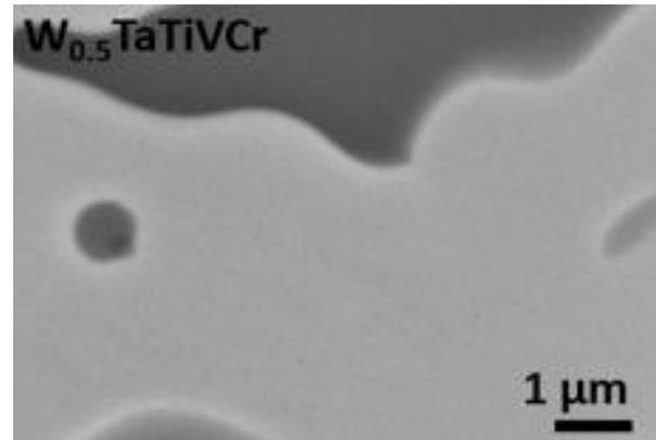
Fig. 1. SEM microstructure of He+ ion irradiated  $W_xTaTiVCr$  sample.
