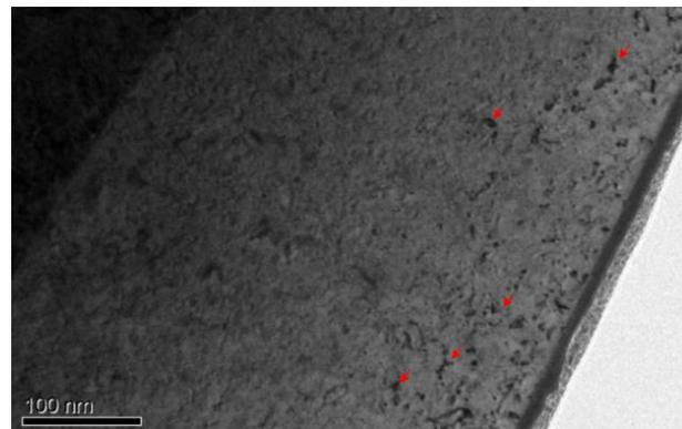
Fig. 2. Representative TEM microstructure of He+ ion irradiated  $W_xTaTiVCr$ .
