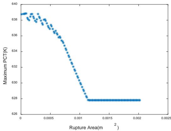
Fig. 12. Highest PCT for different break size - SMR.
