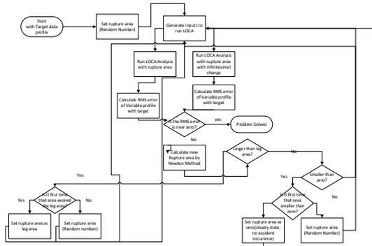
Fig. 3. Algorithm for Initial Condition Tracking System.
