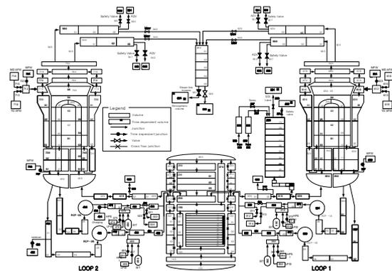
Fig. 1. Nodalization of KSNP for LBLOCA analysis.
