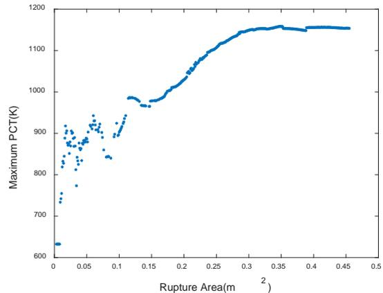
Fig. 10. Highest PCT for different break size – Large PWR.
