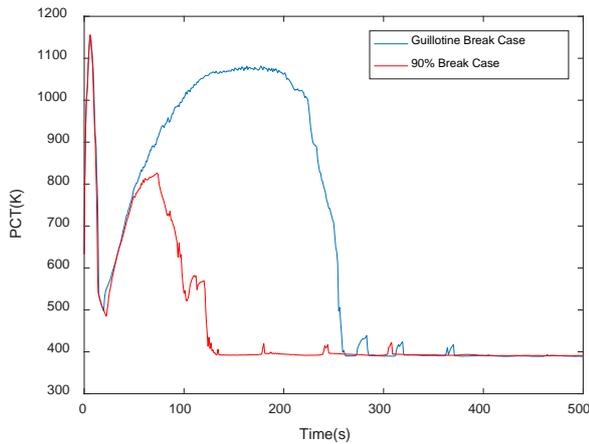
Fig. 11. PCT Profile for selected break size areas in large PWR calculation.
