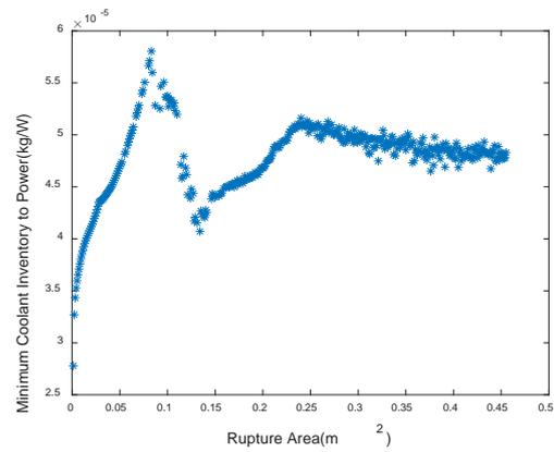
Fig. 13. The minimum coolant inventory to reactor power during problem time - Large PWR
