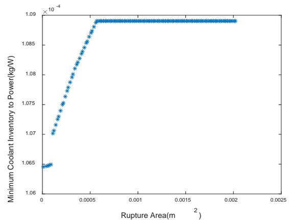
Fig. 14. The minimum coolant inventory to reactor power during problem time - SMR
