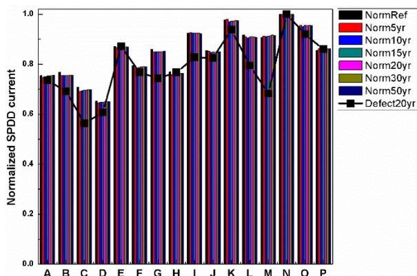
Fig. 9. Modeled current distribution of normal G23 spent fuel assembly (5~50 year cooling) and assembly with partial defects after cooled for 20 years.
