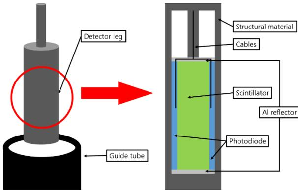
Fig. 3. Design of single SPDD detector leg.
