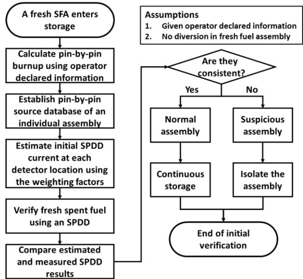
Fig. 1. Flowchart of SPDD based initial spent fuel verification process.
