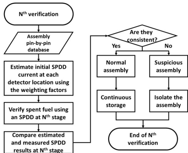
Fig. 2. Flowchart of SPDD based regular inspection process.
