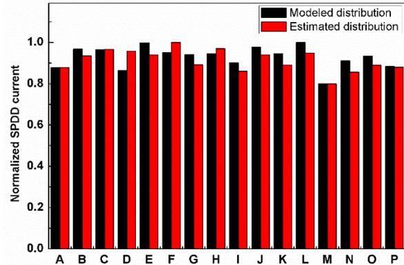
Fig. 6. Estimated and modeled initial current distribution of C15 assembly.
