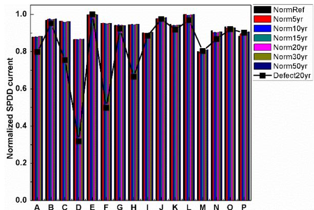
Fig. 8. Modeled current distribution of normal C15 spent fuel assembly (5~50 year cooling) and assembly with partial defects after cooled for 20 years.
