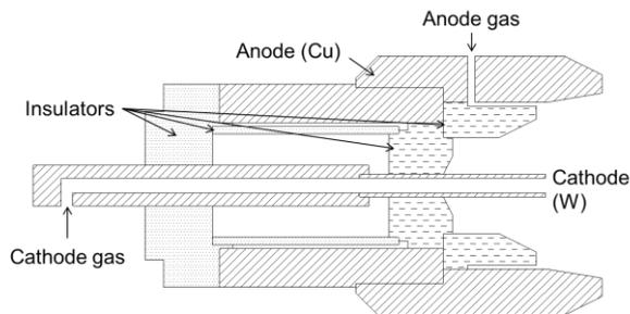
Figure 1. A sketch of our MPD thruster. It consists of Cu anode, W hollow cathode, and three insulating materials. The general concepts are adopted from Ref. [6].
