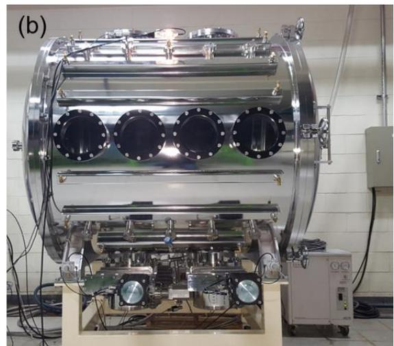
Figure 2. (a) CAD drawing of the vacuum chamber. Chamber is big enough to accommodate the divertor cooling channel mockup. (b) A photo of the vacuum chamber. Two cryopumps are installed at present to provide 5,000 l/s pumping speed.
