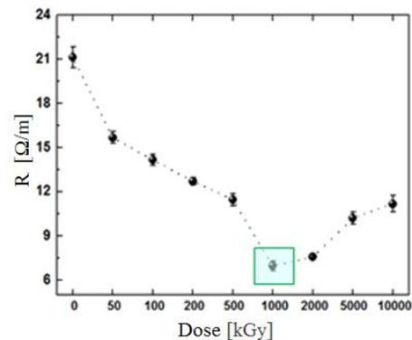
Fig. 1. Resistivity of the CNTs
