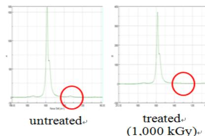
Fig. 2. Raman spectra of CNTs
