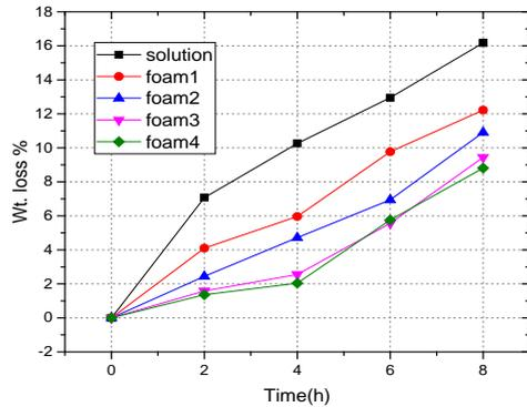
Fig. 1. Weight loss % for the FeCr<sub>2</sub>O<sub>4</sub> specimen in the solution decontaminating agent and foam decontaminating agents.
