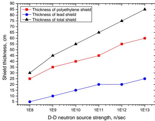
Fig. 6. Minimum shield thickness for various D-D neutron sources
