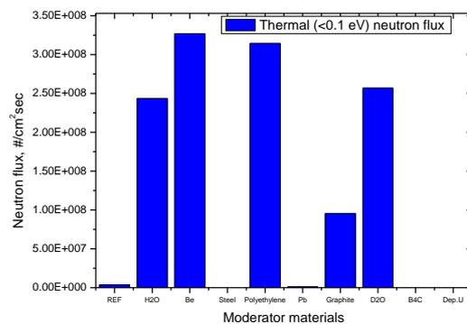
Fig. 2. Thermal neutron fluxes for various moderators
