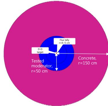
Fig. 1. Approximated 1-D spherical model for conceptual design
