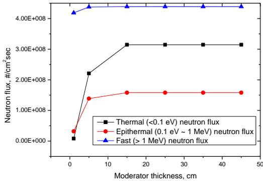
Fig. 3. Thermal neutron fluxes according to the thickness of the polyethylene moderator
