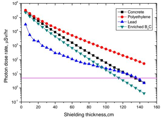
Fig. 5. Photon dose rates for various shield materials
