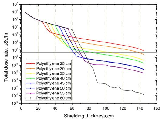
Fig. 6. Total dose rates for combination of polyethylene and lead
