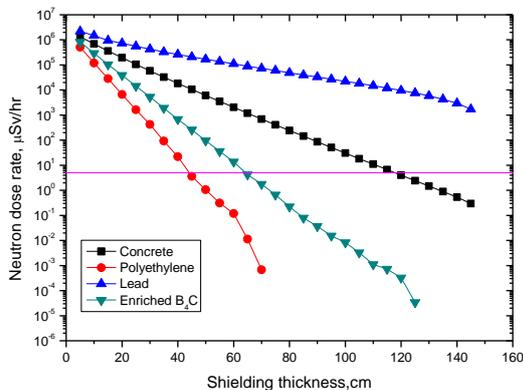
Fig. 4. Neutron dose rates for various shield materials
