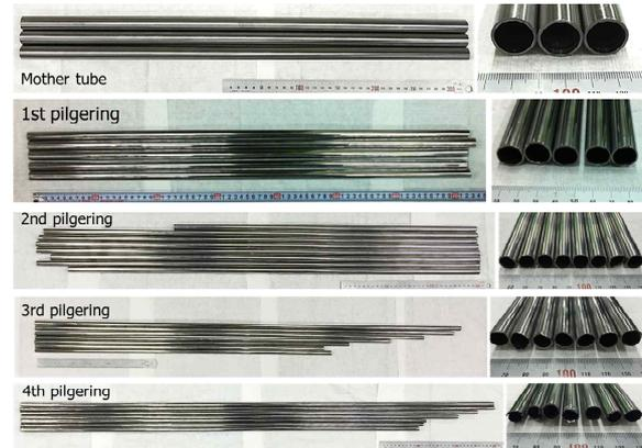
Fig. 3. ARROS tubes fabricated by pilgering process and intermediate heat treatment.
