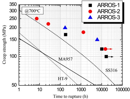
Fig. 2. Creep rupture strengths of ARROS and conventional steels [1].
