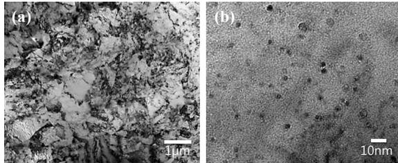
Fig. 1. Microstructures showing (a) grain and (b) nano-oxide morphologies of ARROS [1].
