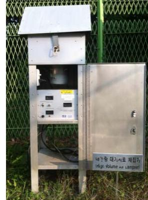
Figure 1: High volume air sampler
