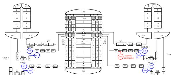
Fig. 1. Pipe model for the reactor simulation
