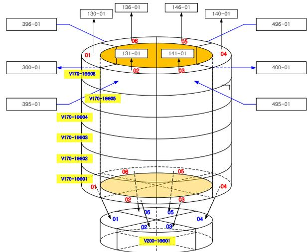
Fig. 3. Downcomer multi-dimensional model for the downcomer
