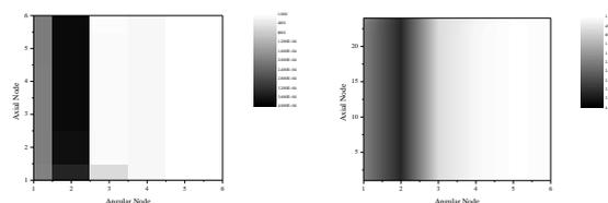
Fig. 7. Mixing behavior of (a) downcomer and (b) core, respectively for the unbalanced flow condition: 100% of loop 1A flow and 90% of loop 1B and 2A, 2B flow of nominal value.
