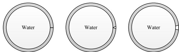
Figure 2. Simple sketch of self-wastage
