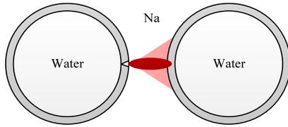
Figure 3. Simple sketch of impingement wastage phenomenon
