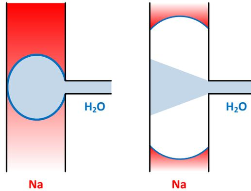
Figure 4. Anticipated flow pattern of SWR in small single tube
