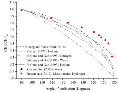
Fig. 3. Normalized CHF according to the angle of inclinations.
