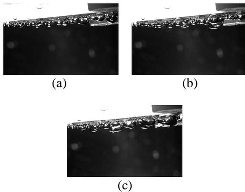
Fig. 6. Vapor behaviors on an inclined surface (175°).
