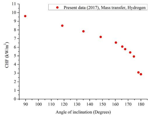
Fig. 2. Absolute CHF value of mass transfer according to the angle of inclination.
