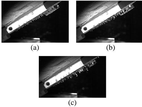
Fig. 5. Vapor behaviors on an inclined surface (150°).
